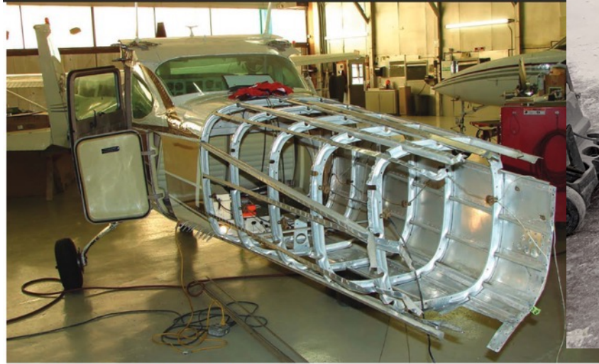
The internal construction of a semi-monocoque airplane showing damage from a wildlife strike.
